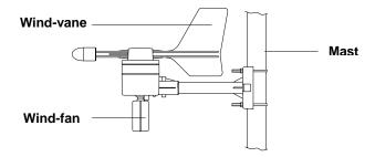
Firstly, check that the wind-fan and the wind-vane can rotate freely before fixing the unit. For correct and accurate readings it is important to mount the sensor so that the front (marked E) is pointing in East-West direction. The wind sensor should now be mounted using the screw provided onto a mast to allow the wind to travel around the sensor unhindered from all directions (ideal mast size should be from  $\emptyset.63^{\circ} - \emptyset1.3^{\circ}$ ).
